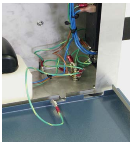
Fig. 4. removing the side panel of the OR 100 organizer rack.
